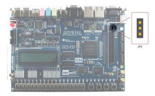
Figure 4-2 The JTAG chain configuration header
