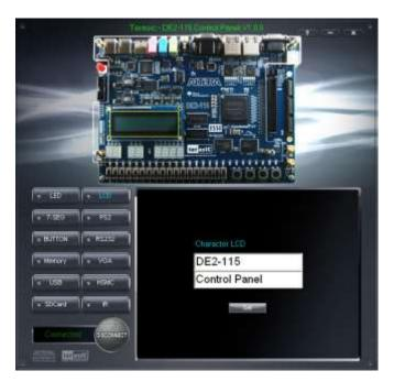
Figure 3-5 Controlling the LCD display
