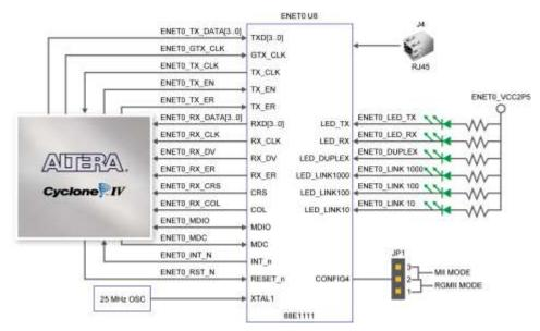
Figure 4-27 Connections between FPGA and Ethernet
