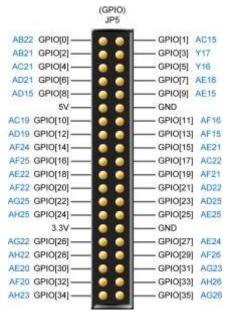
Figure 4-15 GPIO Pin Arrangement
