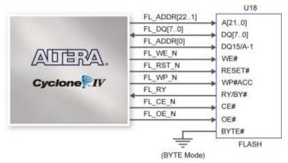
Figure 4-35 Connections between FPGA and Flash
