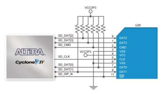
Figure 4-37 Connections between FPGA and SD Card Socket
