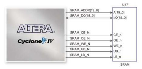
Figure 4-33 Connections between FPGA and SRAM
