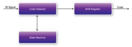
Figure 6-20 The IR Receiver controller
