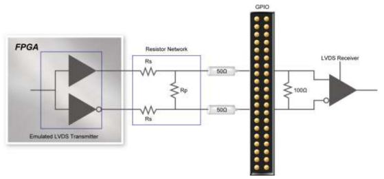
Figure 4-19 Using Emulated LVDS on GPIO
