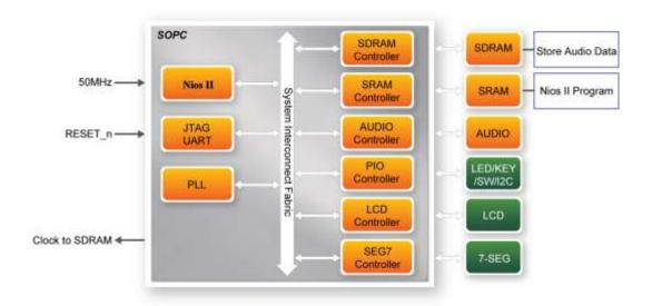
Figure 6-26 Block diagram of the audio recorder and player
