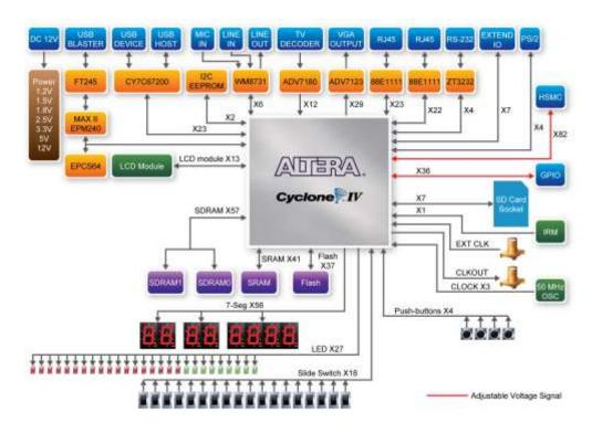
Figure 2-3 Block Diagram of DE2-115
