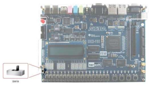
Figure 4-4 The RUN/PROG switch (SW19) is set in JTAG mode
