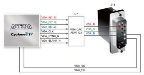
Figure 4-21 Connections between FPGA and VGA
