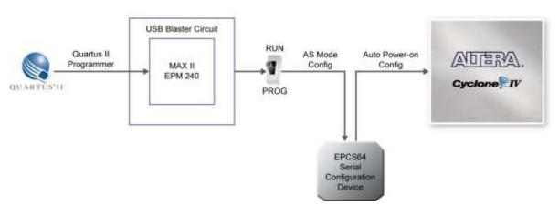
Figure 4-5 The AS configuration scheme
