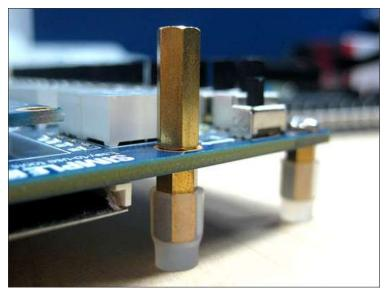
Figure 1-2 The feet for the DE2-115 board
