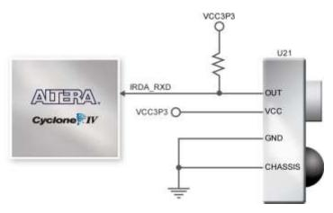
Figure 4-32 Connection between FPGA and IR
