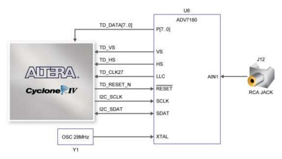
Figure 4-29 Connections between FPGA and TV Decoder
