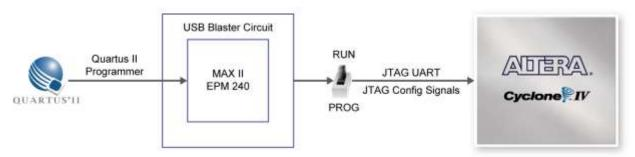
Figure 4-3 The JTAG configuration scheme
