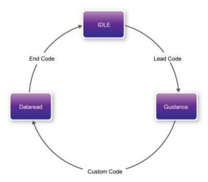
Figure 6-21 State shift diagram of State Machine
