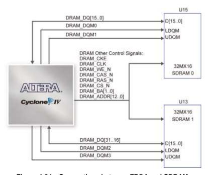
Figure 4-34 Connections between FPGA and SDRAM
