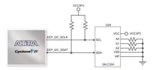
Figure 4-36 Connections between FPGA and EEPROM
