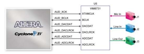
Figure 4-23 Connections between FPGA and Audio CODEC
