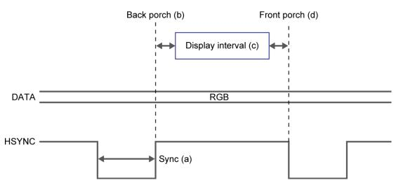
Figure 4-22 VGA horizontal timing specification
