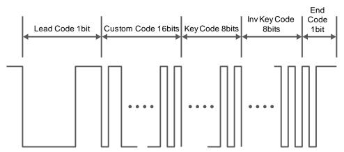
Figure 6-19 The transmitting frame of the IR remote controller
