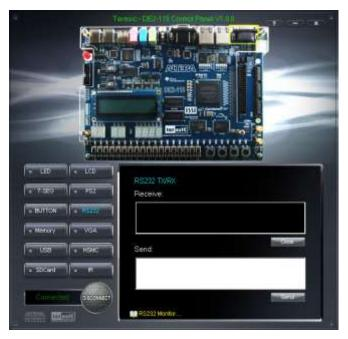
Figure 3-11 RS-232 Serial Communication
