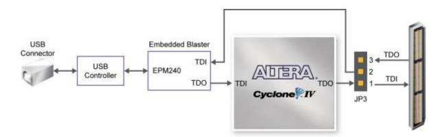
Figure 4-1 The JTAG chain on DE2-115 board
