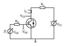
Fig. 6.2.1 Test Circuit of Switching Time
