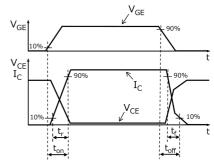
Fig. 6.2.2 Timing Chart of Switching Time
