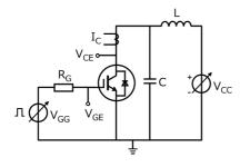
Fig. 6.2.3 Test Circuit of Switching Loss
