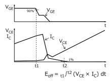
Fig. 6.2.4 Timing Chart of Switching Loss
