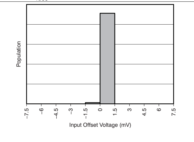
Figure 8. Bus Input Offset Voltage Production Distribution
