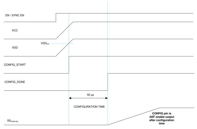
Figure 8-6. Configuration Timing
