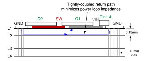
Figure 11-4. PCB Stack-up Diagram With Low L1-L2 Intra-layer Spacing <sup>1</sup>
