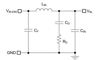
Figure 9-2. Passive π-Stage EMI Filter for Buck Regulator
