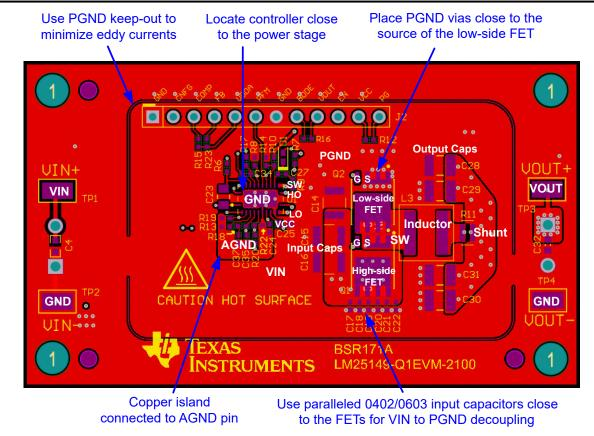
Figure 11-2. PCB Top Layer - High Density, Single-sided Design
