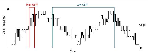
Figure 8-3. Dual Random Spread Spectrum Implementation
