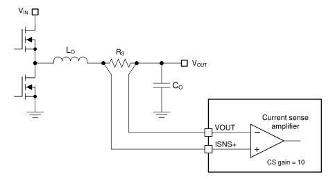
Figure 8-4. Shunt Current Sensing Implementation
