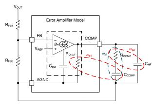
Figure 9-4. Error Amplifier and Compensation Network
