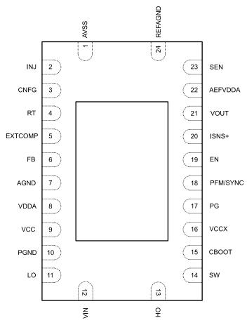
Connect the exposed pad to AGND and PGND on the PCB.
