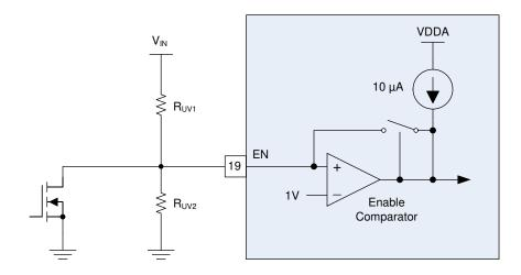
Figure 8-1. Programmable Input Voltage UVLO Turnon
