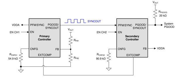
Figure 8-7. Schematic Configured for Single-Output Multi-Phase Operation
