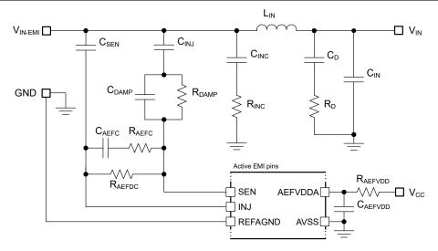
Figure 9-3. Active EMI Filter for a Buck Regulator
