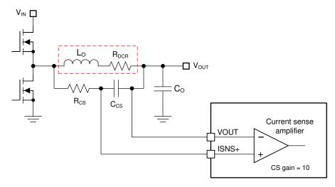
Figure 8-5. Inductor DCR Current Sensing Implementation
