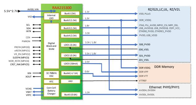
Figure 1. Typical Application Diagram - MPU Power (RZ/G, RZ/V2L)
